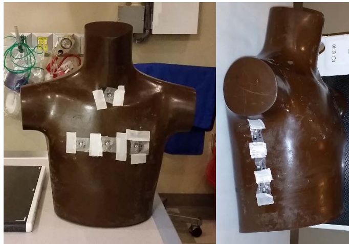
Figure 5-1: Placement of the nanoDot dosimeters on the Alderson chest phantom. 4 nanoDots placed on the anterior and posterior surfaces, 3 nanoDots placed on lateral surfaces.
