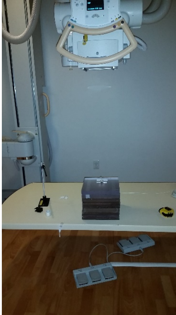
Figure 3-3: 0.6cc ion chamber placed on surface of polystyrene blocks.
