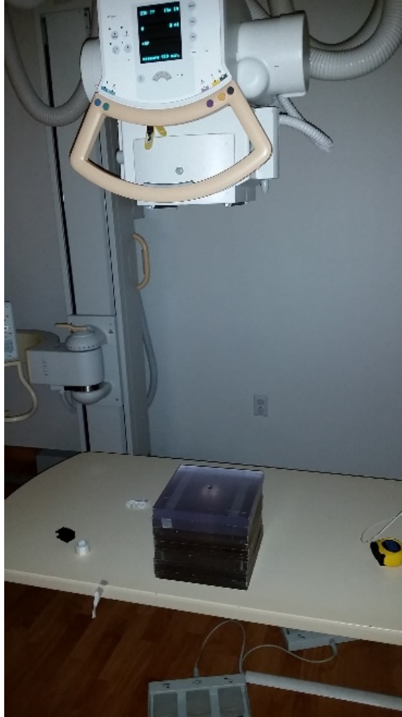
Figure 3-4: nanoDot placement on polystyrene blocks. The rest of the configuration matches the ion chamber setup.
