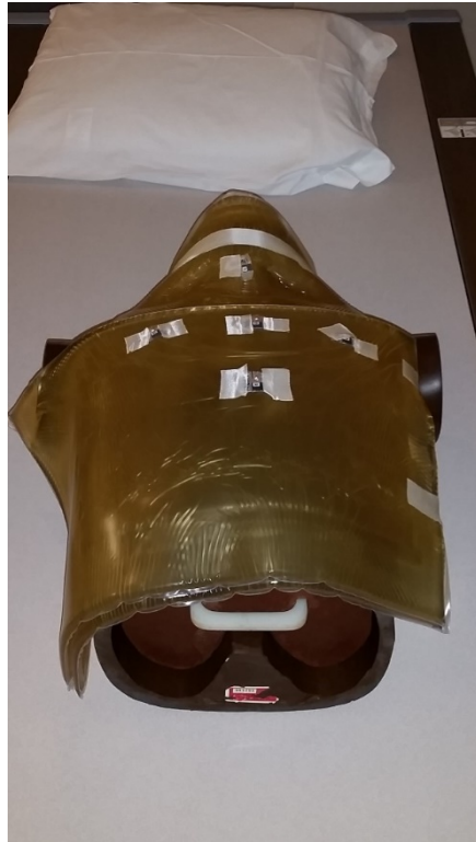
Figure 5-4: Anthropomorphic phantom with 5cm of Super-flex added, and nanoDot dosimeters in place.
